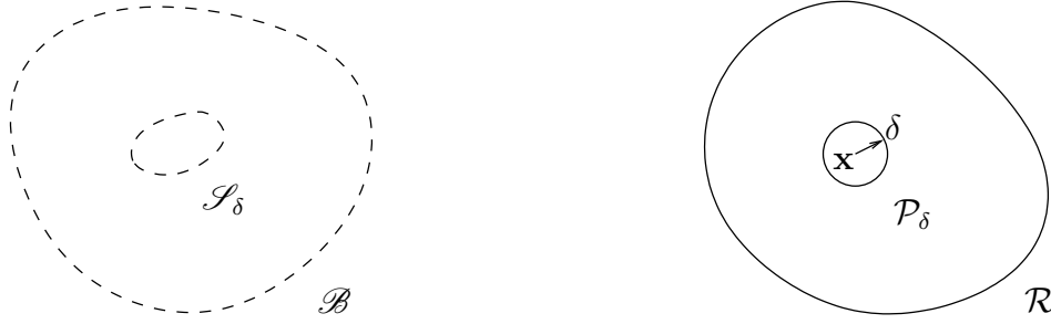
Figure 4.4. A limiting process used to define the mass density \rho at a point \mathbf{x} in the current configuration.
